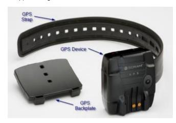
(236 grams), and is sealed and waterproof to two meters. The SCRAM GPS device has been tested and complies with military standards MIL-STD-810F Method 516.6 and IP-57 respectively for shock and water ingress and is FCC compliant (FCC ID P8M-GPS-600).
