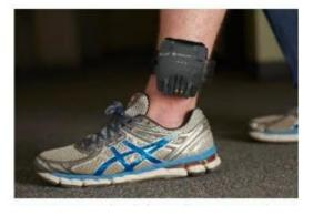
Scram GPS is a slim, lightweight, one-piece device that attaches to the client's ankle and tracks movements 24/7.
